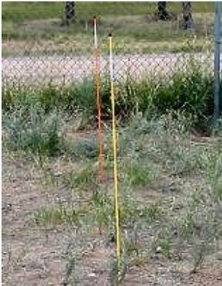
To perform the survey, you set up a plumb bob, or an exactly vertical stake, and mark the shadow at solar noon. Get ready beforehand, and work fast, because the sun doesn't wait around. We set up 2 stakes with a string, planted one stake, and moved the second stake until the string lined up over the shadows. Then we planted the second stake. The two stakes served as our true North-South reference for the foundation.
