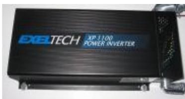
The final component to check out was the inverter. We turned on the 100 Amp inverter breaker, and flipped the power switch. The green LED lit up. Good. We measured the voltage at the convenience outlets on the front panel with a DVM: 120 VAC from hot to neutral; 120 VAC from hot to ground; 0V from neutral to ground. We plugged in a droplight, and that worked. Following
